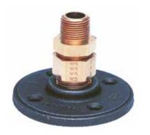
FlashShield™ Termination Fittings are made with cast-iron and galvanized steel, and are able to mount to a floor or wall. They connect and terminate FlashShield™ gas tubing to standard threaded pipes or fittings.
