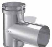
These Ventinox/DuraFlex Tees can be used to transition between liner and connector pipe at the wall thimble, or the rear flue outlet of an appliance. Featuring a 8" long, removable tee snout designed with internal draw bands, allowing for easier, through the wall thimble installations.
