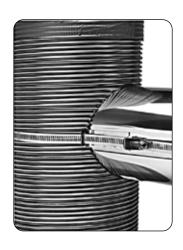
Because of its unique, continuous welded seam, Ventinox VFT Liner is one of the few liner systems in the world that offers the ability to install these Universal Take-Offs directly to the body of the liner. When you drill into Ventinox Liner with a hole saw, we recommend in reverse, it provides a clean cut with no unraveling, allowing the Universal Take-Off o act as a tee snout. The liner must be a minimum of 1" larger
