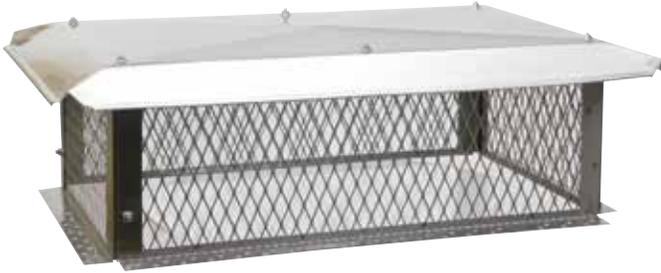
The Premier Top Mount Multi-Flue Cap, made with 304 stainless steel, has a top mount design that is easily attached to the top of the chimney crown or brick with chimney top adhesive and tapcons (included). All Premier Top Mount Multi-Flue Caps have a hinged mounting system (piano hinge), that gives extra space for a tight fit. These caps are great at keeping out animals and debris!
