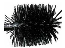
Polypropylene Brushes are constructed of corrosion resistant, .075" polypropylene bristles, set in a single spiral configuration. These stiff bristles make this the best cleaning brush for gas, coal, oil, prefab flues, and chimney liners. Made with a % standard pipe thread end, which connects to standard fiberglass cleaning rods.
