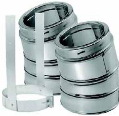
These Offset Elbow Kits for DuraTech chimney pipe are ideal when navigating pipe around obstructions such as rafters, ridgepoles, or joists. These kits provide you with a 16" L x 2" W elbow strap, and two elbows: one for the offset, and one for the return to vertical. These elbows also feature a 360° swivel base
