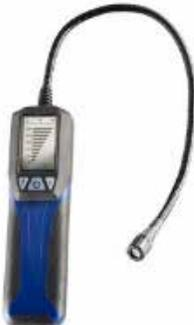
The GS 300 Gas Sniffer from Wöhler is a highly sensitive, and quick responding, gas detection product for leakage detection of gas lines carrying combustible gases. This product features an acoustic signal and vibration alarm to display even the smallest of leaks! Able to detect concentrations from 0 to 1200 ppm, this device is the perfect safety tool when working with natural or liquefied gas installations.
