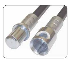
The Torque Lock Connector Rods have a ridge on the top of the rod and a groove in the bottom of the female end. This design provides added security to prevent the rods from separating, and strengthens the joint when using rotary cleaning tools or tile breakers. These TLC connectors also provide a smooth transition joint, preventing it from catching on uneven flue tiles.
