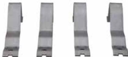
Leg Kits are made with heavy, 11 gauge, 304 stainless steel. They are designed to grip the interior of a chimney flue, holding a cap in place with a unique corner mount attachment. These Leg Kits come in sets of four, and are specifically made to work with the Square, Single Flue, Stainless Steel Caps from HY-C. These leg kits are not designed to work with SmartStack multi-pack caps.
