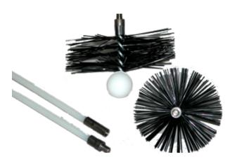
This Pellet/Dryer Vent Brush features quality, nylon bristles, and a guide ball to help prevent snagging. It screws onto Pellet Rods, and is stocked in 3" and 4" diameters. The flexible 4' Pellet/Dryer Vent Rods have a threaded male and female end (1/4" - 20 thread). These are an economical choice for cleaning pellet appliance flues and dryer vent flues, and are for hand brushing only.
