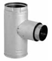
The Increaser Adapter Tee & Cleanout Tee Cap attaches directly to an appliance as an adapter, converting 3" appliance exhausts to 4" PelletVent Pro vent pipe. They are used for 90° offsets, and incorporate a removable, twist-lock Cleanout Tee Cap.
