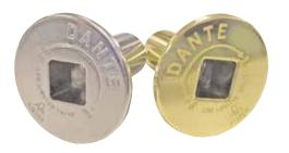
These floor plates are used to stylishly install the Universal Gas Keys, and are available in Brass and Chrome finish. They can be installed on the outside wall of the fireplace or floor. The face plate is 2  $\frac{1}{8}$ " wide, shaft length 2 1/16" long, and shaft width of 1" OD.
