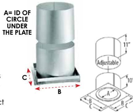
The Firestop Radiation Shield is required for ceiling/floor penetrations when a ceiling support is not used, but is not required for passing through a roof. This shield fits on the ceiling side of the installation and adjusts in height.
