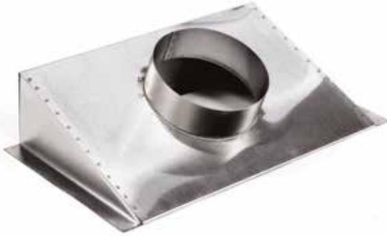
These SmartFlex Insert Boots are 24 gauge, 304 stainless steel, and designed to attach rigid pipe or flexible liner with a coupler to the exhaust vents of most inserts. These insert boots come with a variety of opening sizes, and measure 10" W x 16" L x 4" H.
