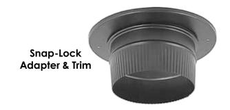
This Snap-Lock Adapter & Trim connects to a ceiling support box, or finishing collar. It extends down to fit into a stovepipe for a drip-free, strong, mechanical connection. This adapter will connect to DuraBlack stovepipe as well as DuraTech, DuraPlus, DuraPlus HTC, or DuraLiner.
