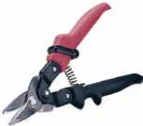
The Malco straight Bull Snips have an 18 gauge capacity for stainless steel, and jaws that are hot-drop forged from high carbon alloy steel and fully heat treated for strength.
