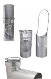
These SmartFlex Two Part Tees are available in 316 or 304 stainless steel, and for use with flex liner (316), or rigid pipe and OD liner (304). The "EZ" band clamp ensures these tees maintain mechanical integrity in extreme heat conditions.
