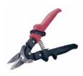
The Malco straight Bull Snips have an 18 gauge capacity for stainless steel, and jaws that are hot-drop forged from high carbon alloy steel and fully heat treated for strength.
