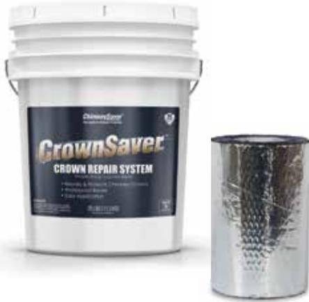
CrownSaver is a strong, cement based, long term crown repair product made with a blend of polymer modified hydraulic cements and powdered water repellent. For best results, cover the crown with FormFoil - a sticky, adhesive-backed, aluminum foil flashing (sold separately). Then, simply mix one scoop CrownSaver (measuring scoop included) with three scoops fine
