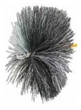
Duct cleaning has become a lucrative add-on business for Chimney Professionals. These Duct Cleaning Brushes have floppy bristles, and are great for cleaning ducts as well as large gas or oil flues. It has a standard 3/8" fitting, and connects to standard fiberglass rods.
