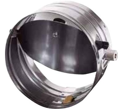
Barometric Dampers allow air to mix with the heated flue gases from furnaces and boilers reducing draft fluctuations creating a more stable combustion of fuel. These dampers are constructed with galvanized steel and must be installed in a tee snout. These dampers provide settings from .02" - .08" of water column.
