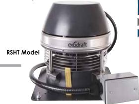
The RSHT Chimney Fan is for use with wood, pellet, or coal applications where flue gas temperatures do not exceed 1400° F for intermittent operation, and 1000° F for continuous operations.
