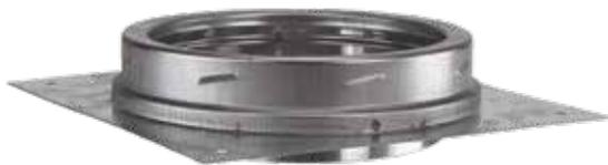
DuraTech Anchor Plates connect directly to a masonry fireplace or a factory-built fireplace that's been listed for use with DuraTech. The plate is galvanized and features a stainless steel, DuraTech twist-lock starter piece. Remember to always check local codes for specifications before installing anchor plates for any chimney system.
