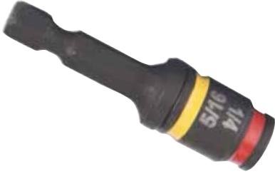
Change between 1/4" and 5/16" hex head sizes seamlessly with Malco's unique, dual-sided magnetic hex driver. This patented, reversible hex socket fits over a 1/4" magnet-tipped, ball locking hex shaft which can be quickly reversed to change sizes. For cleaning, just wipe away metal shavings with a glove or towel.
