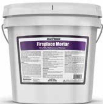
HeatShield® Fireplace Mortar is dry-mix refractory mortar designed for use in indoor residential fireplaces and masonry heaters. Because it is a dry mix, it can be mixed for dipping, grouting, and laying firebrick. After firing (use) the mortar becomes non water soluble. This mortar is extremely sticky and thermal shock resistant with service temperatures tested up to 2550°F (1399°C).
