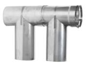
The Double Take-Off Swivel Tee is made with 24 gauge, 316 stainless steel and designed with two take-offs, giving it the capability to spin 360°. This tee features a standard, 2" between take-offs, and comes with an "EZ" band connection.
