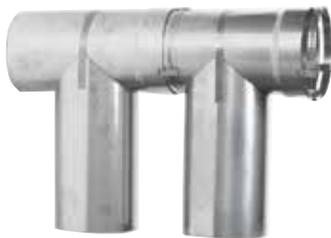
The Double Take-Off Swivel Tee is made with 24 gauge, 316 stainless steel and designed with two take-offs, giving it the capability to spin 360°. This tee features a standard, 2" between take-offs, and comes with an "EZ" band connection.
