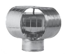
The Vacu-Stack VSS Chimney Cap is a universal, solid pack, factory-built chimney cap used for round, single wall, Class "A", and Type B gas vent chimney pipe. This cap is constructed of 26 gauge, 304 stainless steel and fits into pipe easily. Simply squeeze the base of the cap, slide it into the pipe, and the cap will grip firmly as it expands outwards. The Vacu-Stack VSS Chimney Cap can also be used for masonry chimneys when
