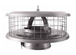
The WeatherShield WSA Chimney Cap is a universal, solid pack, factory-built chimney cap used for round, single wall, Class "A", and Type B gas vent chimney pipe. This cap is constructed of 26 gauge, 304 stainless steel and fits into pipe easily. Simply squeeze the base of the cap, slide it into the pipe, and the cap will grip firmly as it expands outwards. The WeatherShield WSA Chimney Cap can also be used for masonry chimneys when paired with a masonry adapter (sold
