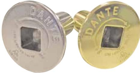
These floor plates are used to stylishly install the Universal Gas Keys, and are available in Brass and Chrome finish. They can be installed on the outside wall of the fireplace or floor. The face plate is 2 1/8" wide, shaft length 2 1/16" long, and shaft width of 1" OD.
