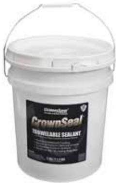
**CrownSeal** is a proprietary elastomeric coating that forms a flexible, waterproof membrane specifically formulated to repair and protect chimney crowns from water intrusion. This thicker material is applied with a trowel and can cover larger cracks in chimney crowns. CrownSeal can be easily colored using standard mortar dye, and covers approximately 36 square feet (2 gal.) or 90 square feet (5 gal.) at 1/8" thickness.
