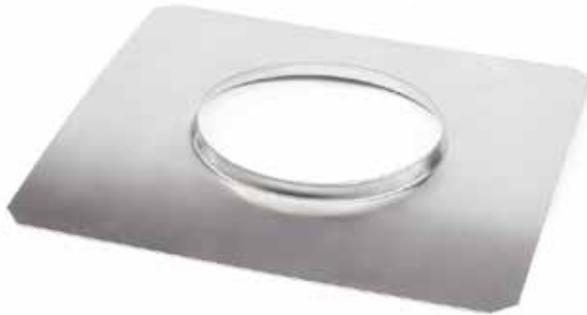
SmartFlex Top Plates are made with 18 gauge, 304 stainless steel which adds extra support when securing the flue pipe. They are available in measurements of 13" x 13" and 18" x 18". These Top Plates also come available with an "EZ" band clamp, which are made with 24 gauge, 304 stainless steel.
