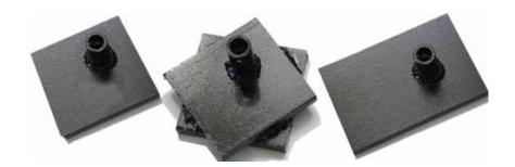
These TLC Tile Breakers easily connect to TLC rods or adapters. Only steel cleaning rods, like the TLC ProKleen Rods, should be used. Use the Small Tile Breaker for 8" x 8" or 7" x 7" flues. For 12" x 12" and larger tiles, use the Large Tile Breaker. The Double Tile Breaker is for 11" x 11" or 8" x 12" flues.
