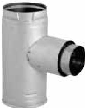
The Increaser Adapter Tee & Cleanout Tee Cap attaches directly to an appliance as an adapter, converting 3" appliance exhausts to 4" PelletVent Pro vent pipe. They are used for 90° offsets, and incorporate a removable, twist-lock Cleanout Tee Cap.
