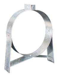
Use these Wall Straps for interior or exterior installations to add support for DuraTech pipe runs! These wall straps are designed to provide 2" - 6" clearance to combustible walls, as well as fit multiple diameters of chimney pipe. DuraTech wall straps are required for every 8' of DuraTech pipe, and come available in either stainless steel or galvanized options.
