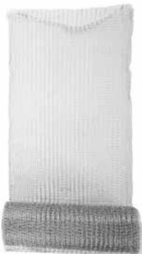
Stainless Steel Mesh protects and permanently holds insulation blankets when installing liner. The mesh, along with a Make-A-Clamp Kit and Stainless Steel Wire, holds the insulation tightly to the liner - minimizing snagging and tearing of the insulation during liner installation. Stainless Steel Mesh is
