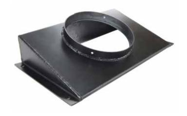
The Round Insert Boots are made with 11 gauge, carbon steel and provide a 20° angle for Ventinox Liner adjustment. Attach the insert to liner with bolts, or by tapping and screwing. The inside base dimensions for this product are  $8 \frac{1}{2}$ " x 16", outside base dimensions are  $10 \frac{1}{4}$ " x 18", with boot height of 4 %".
