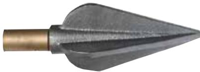
This Boring Tool is great for removing blockages. It features rust-resistant, brass, Universal Threads which connect it to Poly Rods. Always work from below to avoid compacting the blockage.
