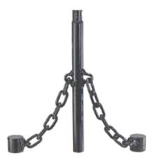
Originally designed and built by a local sweep, these tile breaker tools remove rectangle or square flue tiles faster, and easier than any other on the market today! These tools attach to either the ProKleen, ButtonLok, or TLC rod system, and do not work on round flue tiles.
