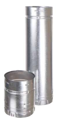
DuraVent Type B Gas Vent Pipe features the DuraLock connecting system, and can be used as a connector, or a standalone vent pipe. This pipe is for use with natural gas fireplaces, gas-fired category I furnaces, boilers, water heaters, and wall or space heating appliances. The recessed, inner wall is .012" aluminum while the outer wall is .018" galvanized and adds 5/8" in wall thickness.
