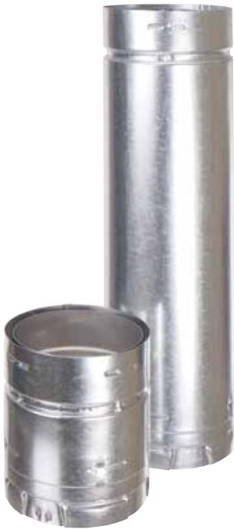
DuraVent Type B Gas Vent Pipe features the DuraLock connecting system, and can be used as a connector, or a standalone vent pipe. This pipe is for use with gas fireplaces, gas-fired category I furnaces, boilers, water heaters, and wall or space heating appliances. The recessed, inner wall is .012" aluminum while the outer wall is .018" galvanized and adds 5/8" in wall thickness.
