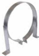
This Wall Thimble for Type B Gas Vent is used when passing pipe through a combustible wall, and can adjust from 3 1/2" - 6" depending on wall thickness. Trim Collars (page 48) can be used in conjunction with the wall thimble as a decorative collar.
