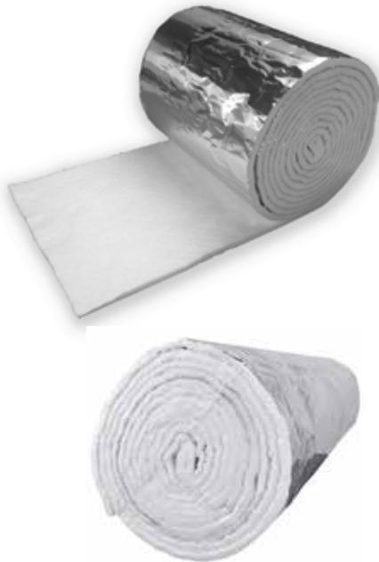
Superwool Plus Insulation Blanket is a non-ceramic, foil-faced, insulation wrap with thick, 3 mil. aluminum facing. It's used as an insulator for stainless steel liners in masonry and wood burning chimneys - usually taking two wraps of 1/4" or one wrap of 1/2". This product has no UL Listing.
