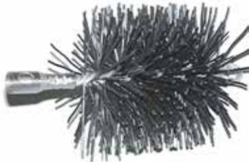
We feature two types of ButtonLok Poly Brushes. The standard ButtonLok Poly Brush is made of .075", single spiral, polypropylene bristles. It is primarily used for factory-built chimneys but can also be used for coal, oil, and gas flues with bristles that are corrosion resistant. The ButtonLok Poly Pro Lite Brush has corrosion resistant bristles for gas, oil, coal, and factory-built chimney flues. The .050" polypropylene bristles on the Poly Pro Lite are wound single spiral on a ButtonLok spine.
