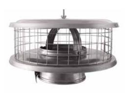
The WeatherShield WSA Chimney Cap is a universal, solid pack, factory-built chimney cap used for round, single wall, Class "A", and Type B gas vent chimney pipe. This cap is constructed of 26 gauge, 304 stainless steel and fits into pipe easily. Simply squeeze the base of the cap, slide it into the pipe, and the cap will grip firmly as it expands outwards. The WeatherShield WSA Chimney Cap can also be used for masonry chimneys when paired with a masonry adapter (sold
