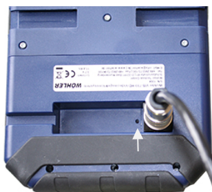
Fig. 52: Reset hole indicated by an arrow
