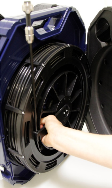
Fig. 57: Grasping the end of the rod and the viper
