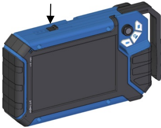
Fig. 15: Push button for pulling out the handle marked with arrow
