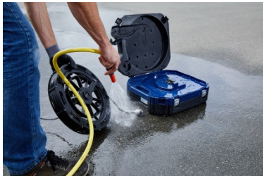
Fig. 60: Cleaning the viper and the rod
