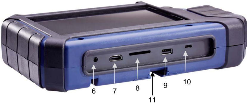
Fig. 8: Bottom side of the monitor with USB and SD card slot
