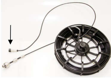
Fig. 59: Viper removed from the case, monitor plug covered by a lid
