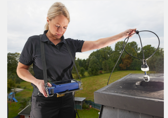
Cable camera: Perfect for inspections from the roof.
