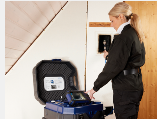
Suitcase camera: Open the case – turn on the camera – start working.
