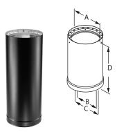
Designed for installation with minimum clearance to combustibles (6" to walls, 8" from top of horizontal run to ceiling). Available in 6", 7", and 8" diameters. Subtract 34" for installed length. Constructed with a stainless steel inner wall.
